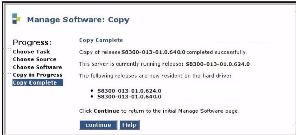
This screen indicates the release just copied, shows the release running on the S8300, and shows the releases resident on the server's hard drive.
