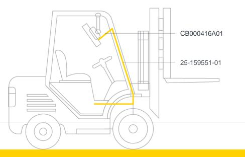
VEHICLE MOUNT (WHEN REPLACING VC70 AND REUSING THE VC70 DC POWER CABLE)
