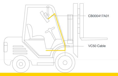
VEHICLE MOUNT (WHEN REPLACING VC50 AND REUSING THE VC50 DC POWER CABLE)
